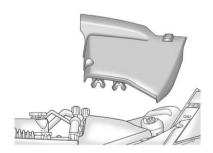
Remove the side cover by pulling up on the front of the cover.
